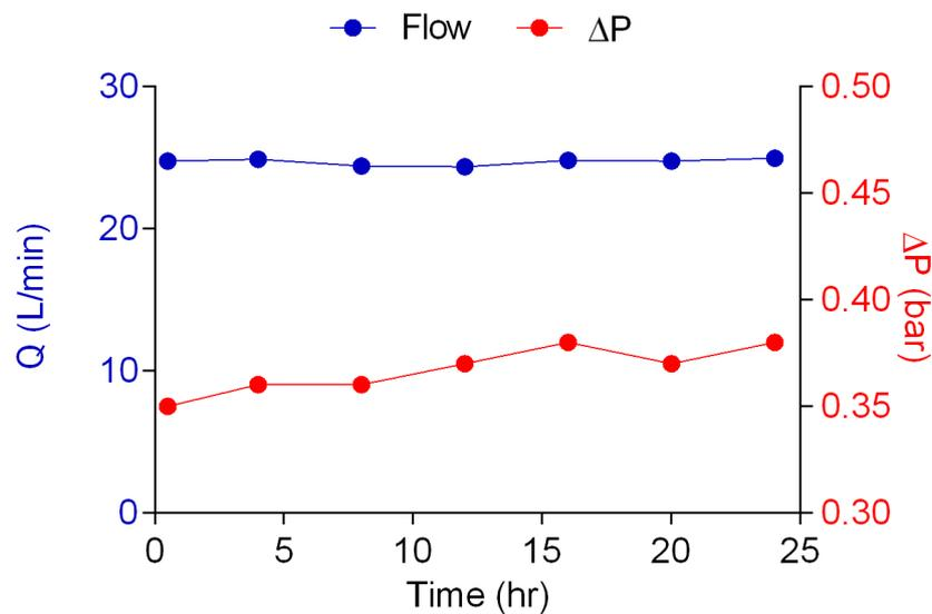
Figure 1. Profile of flow rate (•) and pressure (•) for the Sheaf filter during the pilot at the Nilit plant. Average of phase A and B for a 24 hour cycle.
