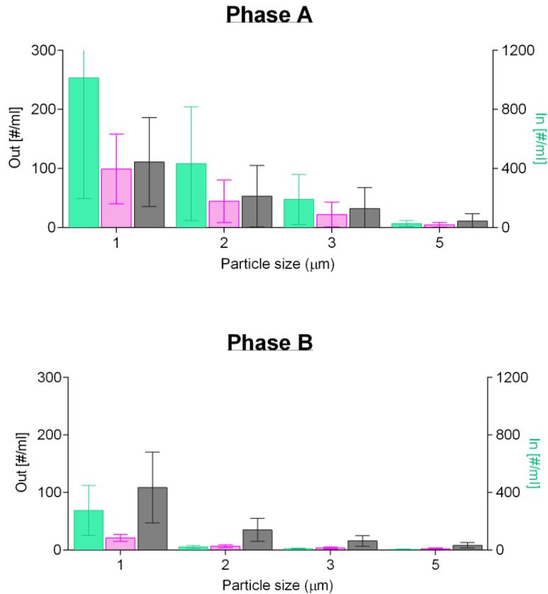
Figure 2. Particle count results for (●) feed and permeate (●) sheaf and (●) reference (ref). Upper panel: phase A where ref=cartridge; Lower panel: phase B where ref= sand + cartridge.
